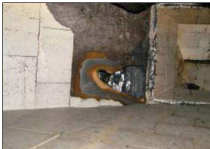
Failure of tile-lined chute after four months prior to patch weld.
